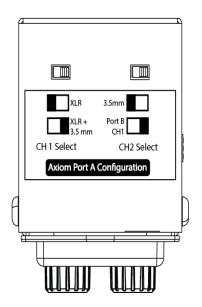
**CH 1 Select:** route either the XLR or a sum of the XLR and 3.5 mm inputs to the CH 1 output of Axiom Port A (on the AXP2O).
