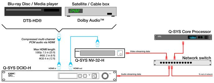
Figure 1 — Connecting the DCIO-H and NV-32-H to de-embed multi-channel audio from an HDMI AV source.
