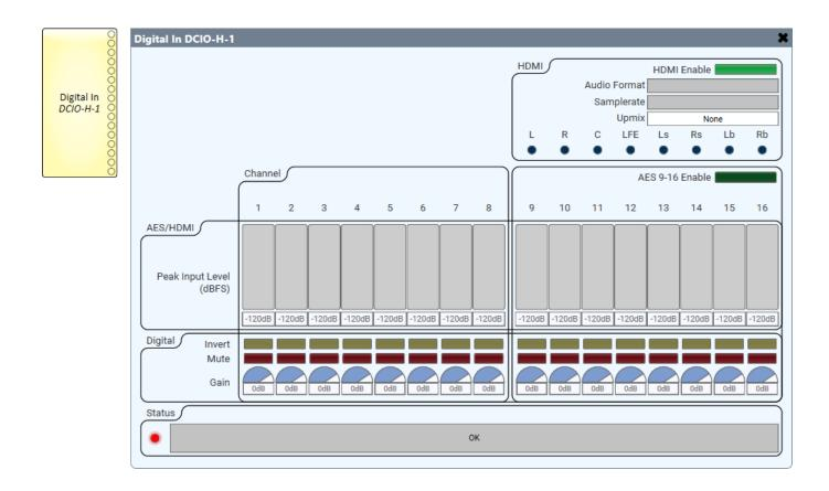
Figure 2 — When enabled, the eight available HDMI audio channels replace AES channels 9 through 16.
